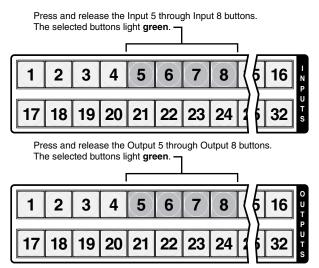
Figure 3-35 — Assign inputs and outputs
